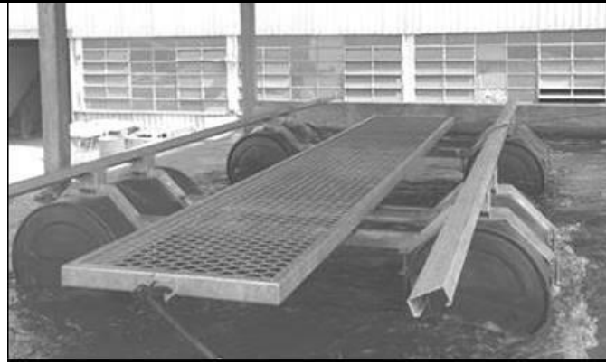
Fig.3: Illustrative picture of the prototype of the flotation module under watertight test and stability over water under conditions of greater turbulence.
